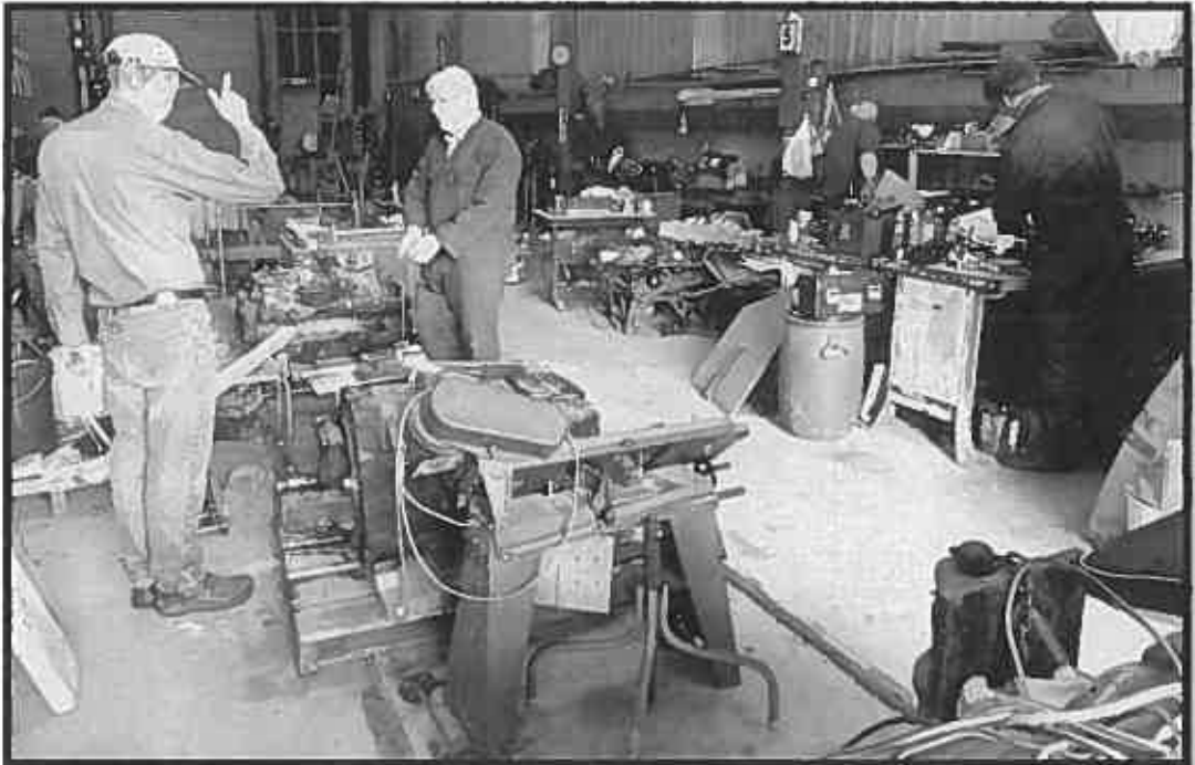
Above: In the workshop, 28 th November 2018. Electric motors for Tram 17 are in the foreground. In the background members are working on tram 17's magnetic brakes and the restoration of a controller.
